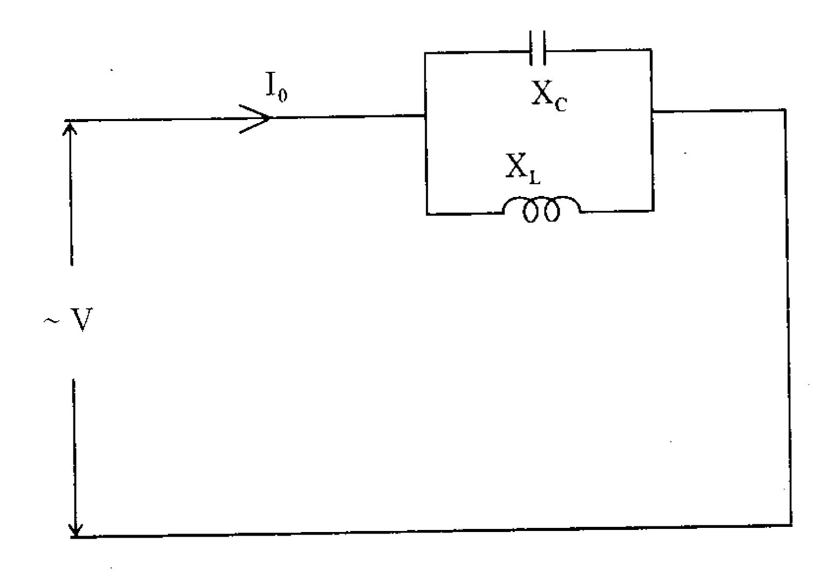
Prove that, under resonant condition, current from source,  $I_{\scriptscriptstyle 0}$ , is zero. Assume ideal  $X_{\scriptscriptstyle C}$  and  $X_{\scriptscriptstyle L}$
